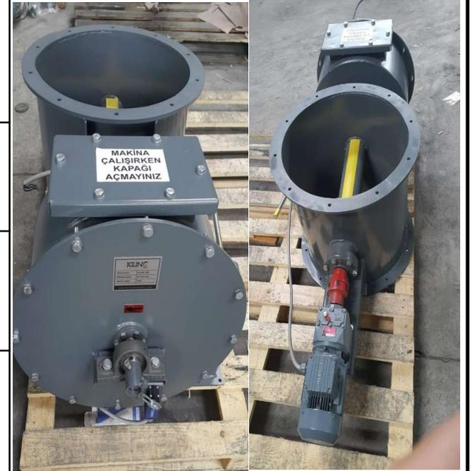
**Manufacturing of 1 screw type sampler to 1 separator
