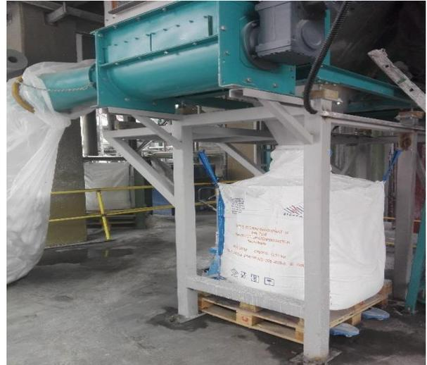
It is used in many industrial facilities as well as cement, mining and chemical plants. Equipment with a maximum capacity of 300 packs/hour is offered to the service of its customers, especially by leak-proof and washable design for the separation of chemical products. Equipment of package shredder;
