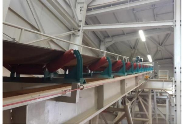
The conveyor belt can be produced from PVC, polyurethane, rubber and mat material depending on the properties of the product to be transported. It is also suitable for the transporting the boxed, bulk and packaged products. Main advantages and equipment of belt conveyors;
